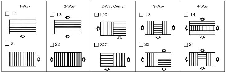
Note: For square diffuser (Height = Width), specify S-1, S-2, etc. Patterns are shown looking at the diffuser face.
